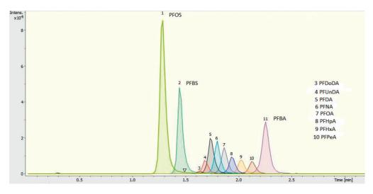
The elimination rates of individual PFAS are determined by LC-MS. The chromatogram shows the retention of PFAS with different chain lengths and functionalities in a raw water sample.
