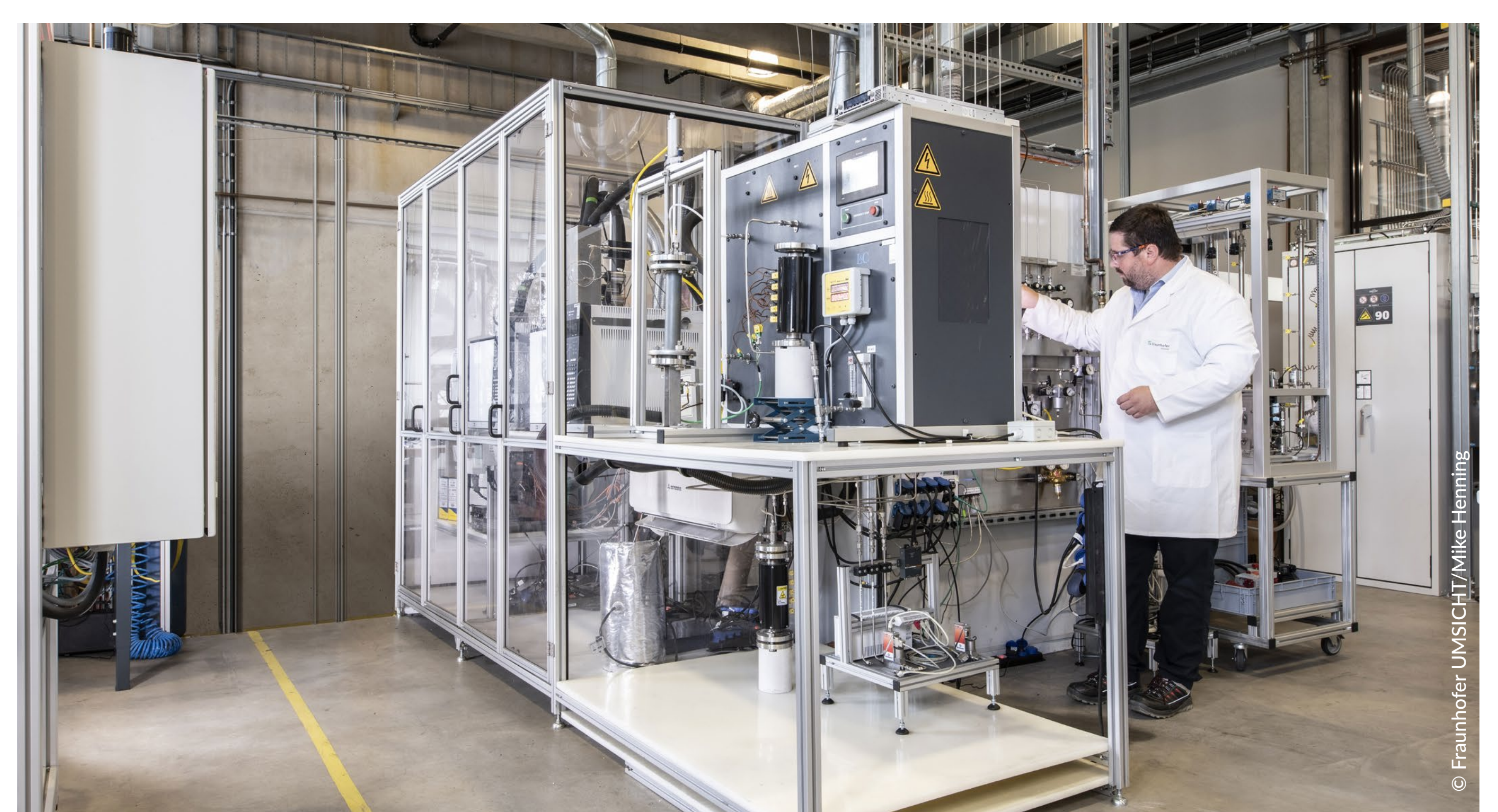
ESA on a laboratory scale with GC system for measuring minor components.
