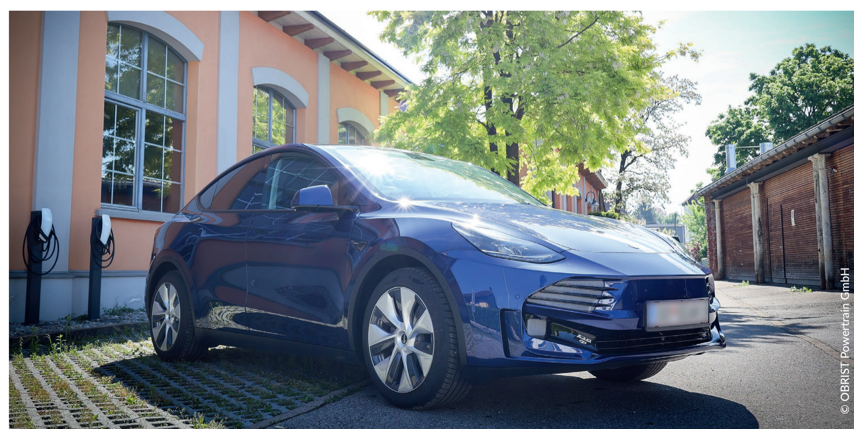
One of 10 prototypes by OBRIST, this Tesla Model Y converted to a plug-in hybrid runs on eMethanol.
